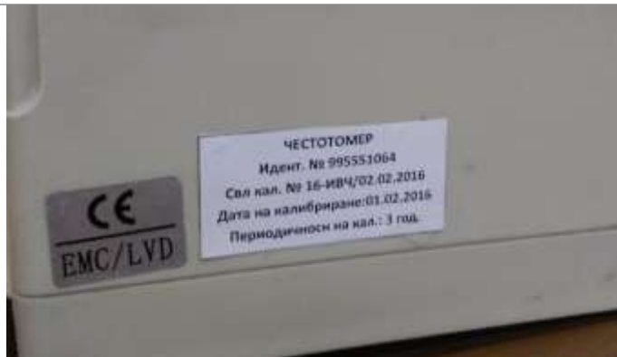
Pic 6 - Calibration identification of Frequency meter
